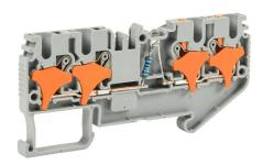
Konnect-It screwless common point feedthrough terminal block, single-level, 2 inputs to 2 outputs bridged with power indicator, accepts wire size 28-12 AWG, gray, 20A, 110 VAC/VDC, LED indicator(s), 35mm DIN rail mount. Package of 25.
