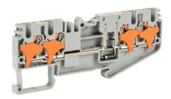
Konnect-It screwless common point feedthrough terminal block, single-level, 2 inputs to 2 outputs bridged with diode, cathode on output, accepts wire size 28-12 AWG, gray, 1A, 300 VAC/VDC, 35mm DIN rail mount. Package of 50.
