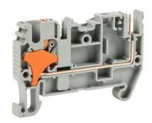
Konnect-It screwless feedthrough terminal block, single-level, pin connection input, accepts wire size 28-12 AWG, gray, 10A, 150 VAC/VDC, 35mm DIN rail mount. Package of 25.
