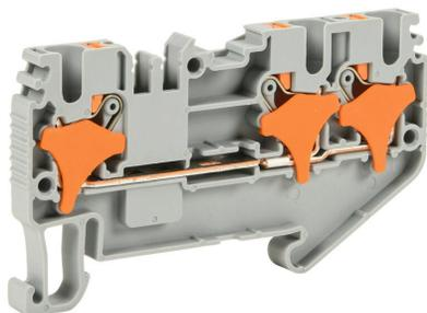
Konnect-It screwless feedthrough terminal block, single-level, 2 inputs to 1 output, accepts wire size 28-12 AWG, gray, 20A, 600 VAC/VDC, 35mm DIN rail mount. Package of 50.
