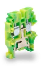
Konnect-It screw mini grounding terminal block, accepts wire size 26-12 AWG, green and yellow, 15mm DIN rail mount, 100kA SCCR. Package of 50. Use to mechanically and electrically connect wires to 15mm DIN rail through the snap-on clamping foot.
