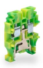
Konnect-It screw mini grounding terminal block, accepts wire size 26-12 AWG, green and yellow, 15mm DIN rail mount, 100kA SCCR. Package of 10. Use to mechanically and electrically connect wires to 15mm DIN rail through the snap-on clamping foot.
