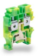
Konnect-It screw mini grounding terminal block, accepts wire size 26-10 AWG, green and yellow, 15mm DIN rail mount, 100kA SCCR. Package of 50. Use to mechanically and electrically connect wires to 15mm DIN rail through the snap-on clamping foot.
