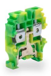
Konnect-It screw mini grounding terminal block, accepts wire size 26-10 AWG, green and yellow, 15mm DIN rail mount, 100kA SCCR. Package of 10. Use to mechanically and electrically connect wires to 15mm DIN rail through the snap-on clamping foot.
