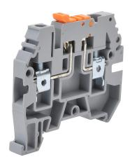
Konnect-It screw disconnect terminal block, accepts wire size 26-10 AWG, gray, 16A, 35mm DIN rail mount, 10kA SCCR. Package of 50.
