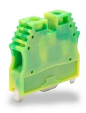
Konnect-It screw grounding terminal block, accepts wire size 16-8 AWG, green and yellow, 35mm DIN rail mount, 100kA SCCR. Package of 25. Use to mechanically and electrically connect wires to 35mm DIN rail through the screw-down clamping foot.
