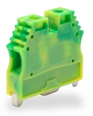
Konnect-It screw grounding terminal block, accepts wire size 16-8 AWG, green and yellow, 35mm DIN rail mount, 100kA SCCR. Package of 10. Use to mechanically and electrically connect wires to 35mm DIN rail through the screw-down clamping foot.
