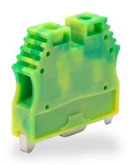
Konnect-It screw grounding terminal block, accepts wire size 16-8 AWG, green and yellow, 35mm DIN rail mount, 100kA SCCR. Package of 10. Use to mechanically and electrically connect wires to 35mm DIN rail through the screw-down clamping foot.
