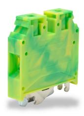
Konnect-It screw grounding terminal block, accepts wire size 12-4 AWG, green and yellow, 35mm DIN rail mount, 100kA SCCR. Package of 50. Use to mechanically and electrically connect wires to 35mm DIN rail through the screw-down clamping foot.
