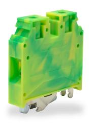
Konnect-It screw grounding terminal block, accepts wire size 12-4 AWG, green and yellow, 35mm DIN rail mount, 100kA SCCR. Package of 10. Use to mechanically and electrically connect wires to 35mm DIN rail through the screw-down clamping foot.
