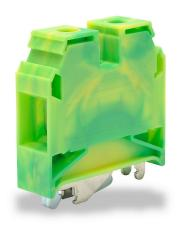
Konnect-It screw grounding terminal block, accepts wire size 12-2 AWG, green and yellow, 35mm DIN rail mount, 100kA SCCR. Package of 40. Use to mechanically and electrically connect wires to 35mm DIN rail through the screw-down clamping foot.
