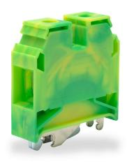
Konnect-It screw grounding terminal block, accepts wire size 12-2 AWG, green and yellow, 35mm DIN rail mount, 100kA SCCR. Package of 10. Use to mechanically and electrically connect wires to 35mm DIN rail through the screw-down clamping foot.
