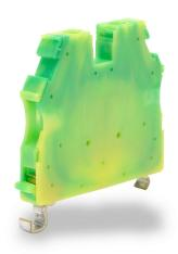
Konnect-It screw grounding terminal block, accepts wire size 26-12 AWG, green and yellow, 35mm DIN rail mount, 100kA SCCR. Package of 50. Use to mechanically and electrically connect wires to 35mm DIN rail through the snap-on clamping foot.
