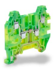
Konnect-It screw grounding terminal block, accepts wire size 26-12 AWG, green and yellow, 35mm DIN rail mount, 100kA SCCR. Package of 25. Use to mechanically and electrically connect wires to 35mm DIN rail through the snap-on clamping foot.
