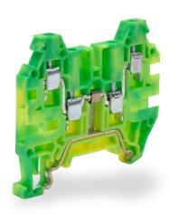
Konnect-It screw grounding terminal block, accepts wire size 26-12 AWG, green and yellow, 35mm DIN rail mount, 100kA SCCR. Package of 10. Use to mechanically and electrically connect wires to 35mm DIN rail through the snap-on clamping foot.
