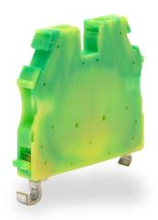
Konnect-It screw grounding terminal block, accepts wire size 26-12 AWG, green and yellow, 35mm DIN rail mount, 100kA SCCR. Package of 10. Use to mechanically and electrically connect wires to 35mm DIN rail through the snap-on clamping foot.
