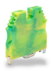
Konnect-It screw grounding terminal block, accepts wire size 26-10 AWG, green and yellow, 35mm DIN rail mount, 100kA SCCR. Package of 50. Use to mechanically and electrically connect wires to 35mm DIN rail through the screw-down clamping foot.
