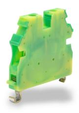
Konnect-It screw grounding terminal block, accepts wire size 26-10 AWG, green and yellow, 35mm DIN rail mount, 100kA SCCR. Package of 50. Use to mechanically and electrically connect wires to 35mm DIN rail through the snap-on clamping foot.
