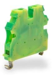
Konnect-It screw grounding terminal block, accepts wire size 26-10 AWG, green and yellow, 35mm DIN rail mount, 100kA SCCR. Package of 10. Use to mechanically and electrically connect wires to 35mm DIN rail through the snap-on clamping foot.
