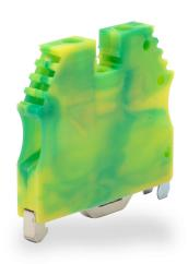
Konnect-It screw grounding terminal block, accepts wire size 26-10 AWG, green and yellow, 35mm DIN rail mount, 100kA SCCR. Package of 10. Use to mechanically and electrically connect wires to 35mm DIN rail through the screw-down clamping foot.
