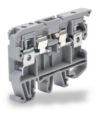
Konnect-It screw circuit protection terminal block, accepts wire size 26-8 AWG, gray, 6.3A, 35mm DIN rail mount, 10kA SCCR. Package of 50. For use with GMA, GMC, S500 and S506 series fuses.
