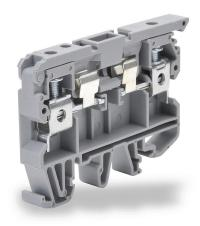
Konnect-It screw circuit protection terminal block, accepts wire size 26-8 AWG, gray, 6.3A, 35mm DIN rail mount, 10kA SCCR. Package of 50. For use with GMA, GMC, S500 and S506 series fuses.
