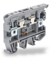
Konnect-It screw circuit protection terminal block, blown fuse indicator, accepts wire size 26-8 AWG, gray, 6.3A, 24 VDC LED indicator(s), 35mm DIN rail mount, 10kA SCCR. Package of 25. For use with GMA, GMC, S500 and S506 series fuses.
