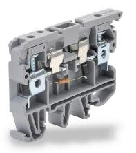
Konnect-It screw circuit protection terminal block, blown fuse indicator, accepts wire size 26-8 AWG, gray, 6.3A, 24 VAC LED indicator(s), 35mm DIN rail mount, 10kA SCCR. Package of 25. For use with GMA, GMC, S500 and S506 series fuses.
