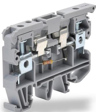
Konnect-It screw circuit protection terminal block, blown fuse indicator, accepts wire size 26-8 AWG, gray, 6.3A, 24 VAC LED indicator(s), 35mm DIN rail mount, 10kA SCCR. Package of 25. For use with GMA, GMC, S500 and S506 series fuses.
