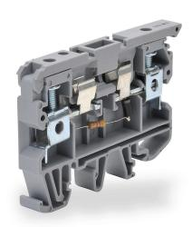
Konnect-It screw circuit protection terminal block, blown fuse indicator, accepts wire size 26-8 AWG, gray, 6.3A, 24 VAC LED indicator(s), 35mm DIN rail mount, 10kA SCCR. Package of 10. For use with GMA, GMC, S500 and S506 series fuses.
