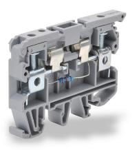
Konnect-It screw circuit protection terminal block, blown fuse indicator, accepts wire size 26-8 AWG, gray, 6.3A, 220 VDC LED indicator(s), 35mm DIN rail mount, 10kA SCCR. Package of 25. For use with GMA, GMC, S500 and S506 series fuses.
