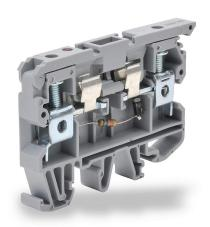
Konnect-It screw circuit protection terminal block, blown fuse indicator, accepts wire size 26-8 AWG, gray, 6.3A, 220 VAC LED indicator(s), 35mm DIN rail mount, 10kA SCCR. Package of 25. For use with GMA, GMC, S500 and S506 series fuses.
