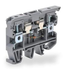
Konnect-It screw circuit protection terminal block, blown fuse indicator, accepts wire size 26-8 AWG, gray, 6.3A, 220 VAC LED indicator(s), 35mm DIN rail mount, 10kA SCCR. Package of 10. For use with GMA, GMC, S500 and S506 series fuses.
