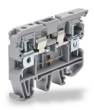
Konnect-It screw circuit protection terminal block, blown fuse indicator, accepts wire size 26-8 AWG, gray, 6.3A, 110 VDC LED indicator(s), 35mm DIN rail mount, 10kA SCCR. Package of 25. For use with GMA, GMC, S500 and S506 series fuses.
