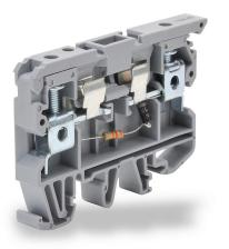
Konnect-It screw circuit protection terminal block, blown fuse indicator, accepts wire size 26-8 AWG, gray, 6.3A, 110 VAC LED indicator(s), 35mm DIN rail mount, 10kA SCCR. Package of 25. For use with GMA, GMC, S500 and S506 series fuses.
