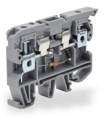
Konnect-It screw circuit protection terminal block, blown fuse indicator, accepts wire size 26-8 AWG, gray, 6.3A, 110 VAC LED indicator(s), 35mm DIN rail mount, 10kA SCCR. Package of 10. For use with GMA, GMC, S500 and S506 series fuses.
