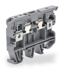
Konnect-It screw circuit protection terminal block, accepts wire size 26-8 AWG, gray, 6.3A, 35mm DIN rail mount, 10kA SCCR. Package of 10. For use with GMA, GMC, S500 and S506 series fuses.
