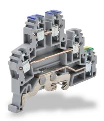
Konnect-It screw double-level feedthrough terminal block, with ground, accepts wire size 26-12 AWG, gray, 20A, 35mm DIN rail mount, 100kA SCCR. Package of 20. For use with jumpers KN-2JTL12, KN-3JTL12, KN-4JTL12 and KN-10JTL12.
