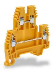
Konnect-It screw double-level feedthrough terminal block, accepts wire size 26-12 AWG, yellow, 20A, 35mm DIN rail mount, 100kA SCCR. Package of 100. For use with jumpers KN-2J12, KN-3J12, KN-4J12 and KN-10J12.
