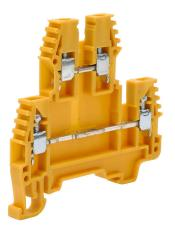
Konnect-It screw double-level feedthrough terminal block, accepts wire size 26-12 AWG, yellow, 20A, 35mm DIN rail mount, 100kA SCCR. Package of 25. For use with jumpers KN-2J12, KN-3J12, KN-4J12 and KN-10J12.
