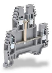
Konnect-It screw double-level feedthrough terminal block, connected between levels, accepts wire size 26-12 AWG, gray, 20A, 35mm DIN rail mount, 100kA SCCR. Package of 20. For use with jumpers KN-2J12, KN-3J12, KN-4J12 and KN-10J12.
