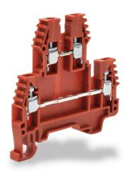
Konnect-It screw double-level feedthrough terminal block, accepts wire size 26-12 AWG, red, 20A, 35mm DIN rail mount, 100kA SCCR. Package of 100. For use with jumpers KN-2J12, KN-3J12, KN-4J12 and KN-10J12.
