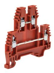
Konnect-It screw double-level feedthrough terminal block, accepts wire size 26-12 AWG, red, 20A, 35mm DIN rail mount, 100kA SCCR. Package of 25. For use with jumpers KN-2J12, KN-3J12, KN-4J12 and KN-10J12.
