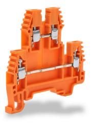
Konnect-It screw double-level feedthrough terminal block, accepts wire size 26-12 AWG, orange, 20A, 35mm DIN rail mount, 100kA SCCR. Package of 100. For use with jumpers KN-2J12, KN-3J12, KN-4J12 and KN-10J12.
