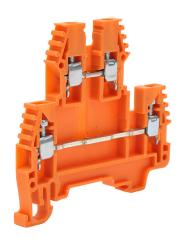
Konnect-It screw double-level feedthrough terminal block, accepts wire size 26-12 AWG, orange, 20A, 35mm DIN rail mount, 100kA SCCR. Package of 25. For use with jumpers KN-2J12, KN-3J12, KN-4J12 and KN-10J12.
