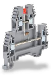
Konnect-It screw double-level feedthrough terminal block, connected between levels and power indicator, accepts wire size 26-12 AWG, gray, 20A, 24 VDC LED indicator(s), 35mm DIN rail mount, 100kA SCCR. Package of 20.
