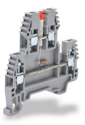
Konnect-It screw double-level feedthrough terminal block, connected between levels and power indicator, accepts wire size 26-12 AWG, gray, 20A, 110 VDC LED indicator(s), 35mm DIN rail mount, 100kA SCCR. Package of 20.
