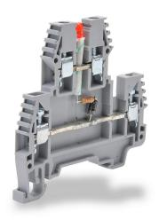
Konnect-It screw double-level feedthrough terminal block, connected between levels and power indicator, accepts wire size 26-12 AWG, gray, 20A, 110 VAC LED indicator(s), 35mm DIN rail mount, 100kA SCCR. Package of 20.
