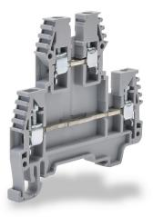
Konnect-It screw double-level feedthrough terminal block, accepts wire size 26-12 AWG, gray, 20A, 35mm DIN rail mount, 100kA SCCR. Package of 100. For use with jumpers KN-2J12, KN-3J12, KN-4J12 and KN-10J12.
