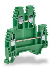
Konnect-It screw double-level feedthrough terminal block, accepts wire size 26-12 AWG, green, 20A, 35mm DIN rail mount, 100kA SCCR. Package of 100. For use with jumpers KN-2J12, KN-3J12, KN-4J12 and KN-10J12.
