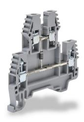
Konnect-It screw double-level feedthrough terminal block, connected between levels and diode, accepts wire size 26-12 AWG, gray, 20A, 35mm DIN rail mount, 100kA SCCR. Package of 20. For use with jumpers KN-2J12, KN-3J12, KN-4J12 and KN-10J12.
