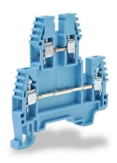
Konnect-It screw double-level feedthrough terminal block, accepts wire size 26-12 AWG, blue, 20A, 35mm DIN rail mount, 100kA SCCR. Package of 100. For use with jumpers KN-2J12, KN-3J12, KN-4J12 and KN-10J12.
