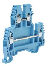
Konnect-It screw double-level feedthrough terminal block, accepts wire size 26-12 AWG, blue, 20A, 35mm DIN rail mount, 100kA SCCR. Package of 25. For use with jumpers KN-2J12, KN-3J12, KN-4J12 and KN-10J12.
